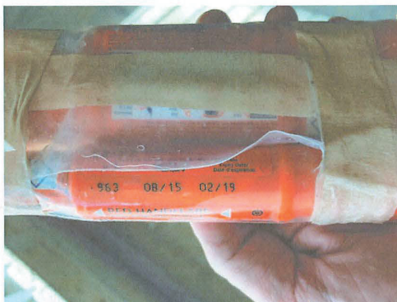
Figure 09. Photograph of recovered life raft expired red handheld flare. Taken by [REDACTED] on October 27, 2022.
